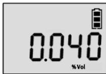
When activated, in Measuring mode, gas concentration is displayed.
