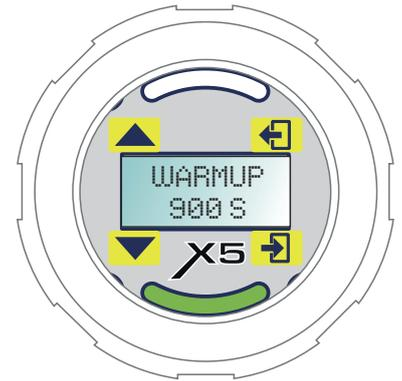
During warm up information is displayed to show the setup of the X5. If two channels are fitted information is displayed sequentially.
