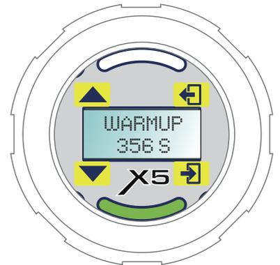
If addressable mode is active then the base address for the unit is also displayed sequentially. The display then indicates the warm up time, this is variable depending on the detector type. After the warm up time the display sequentially shows each detector and its readings.
