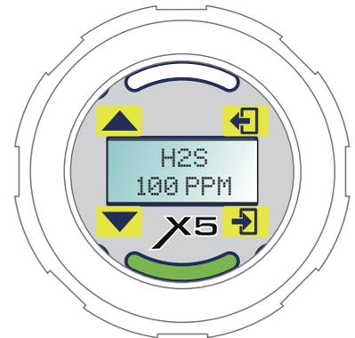
The status indicator stays green if the gas detectors are connected otherwise a channel fault is indicated for the affected channel. The display shows the number of channels and then their type and range.
